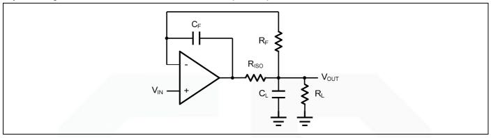
Figure 3. Indirectly Driving a Capacitive Load with DC Accuracy
