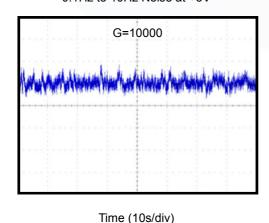
0.1Hz to 10Hz Noise at +2.5V
