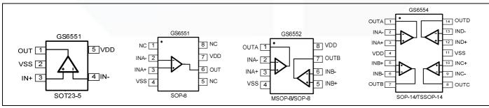
Figure 1. Pin Assignment Diagram
