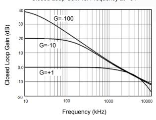
Closed Loop Gain vs. Frequency at +2.5V
