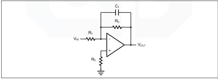
Figure 5. Low Pass Active Filter
