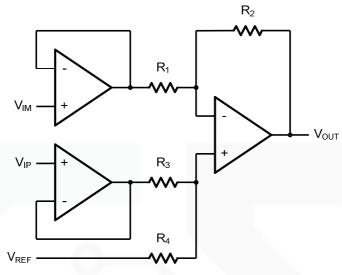
Figure 6. Instrument Amplifier
