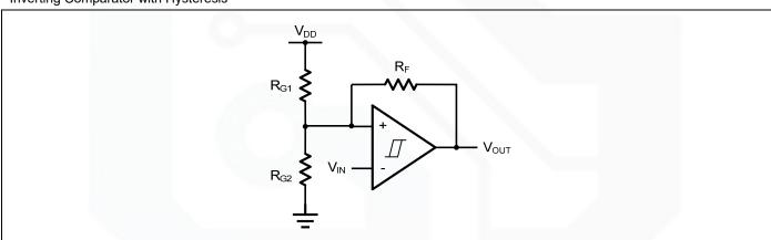
Figure 3. Inverting Comparator with Hysteresis
