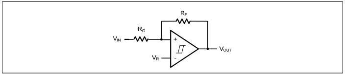
Figure 2. Non-Inverting Comparator with Hysteresis
