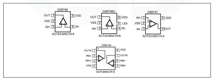
Figure 1. Pin Assignment Diagram
