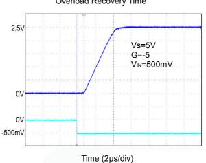
At  $T_A$ =+25°C,  $V_S$ =+5V, and  $R_L$ =100K $\Omega$  connected to  $V_S$ /2, unless otherwise noted. Overload Recovery Time
