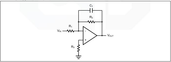
Figure 5. Low Pass Active Filter
