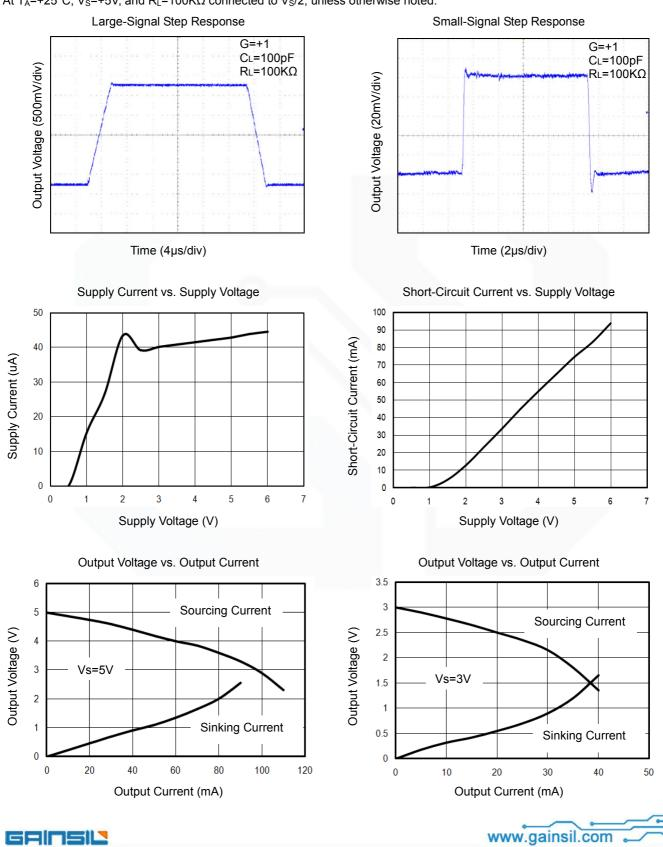
At  $T_A$ =+25°C,  $V_S$ =+5V, and  $R_L$ =100K $\Omega$  connected to  $V_S/2$ , unless otherwise noted.
