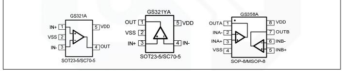
Figure 1. Pin Assignment Diagram
